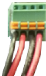
Figure 5-20: Wires Inserted in Terminal Block
